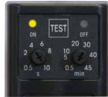
Bright LED illumination, indicating operating status
