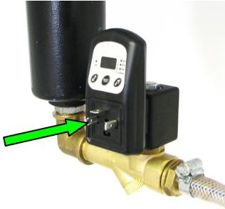
5. Place the connector gasket on the connector and plug the connector on to the timer as illustrated below and tighten the screw (max. 1Nm). Make sure both gaskets are secured properly to ensure IP65 rating.
