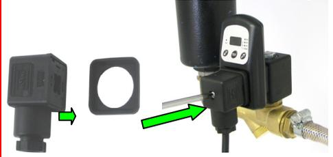
6. After double checking that the power supply corresponds with the voltage specified on the coil and falls within the range specified on the back of the timer, you can switch the power supply ON.
