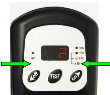
11. To change the ON time, simply press the right 'on/arrow up' button and 'on' will appear briefly on the display.
