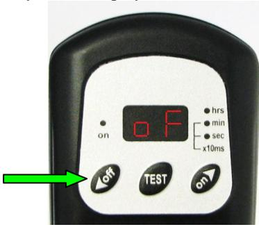
15. You can now press the left 'off/arrow down' button for decreasing the time or the right 'on/arrow up' button to increase the time.
