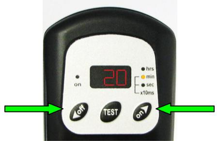
16. If the desired OFF time is set, then simply don't press any buttons and after a few seconds the display will start flashing illustrating that the new time is being saved. Once the new time is saved, the unit will start operating with the new time settings.
