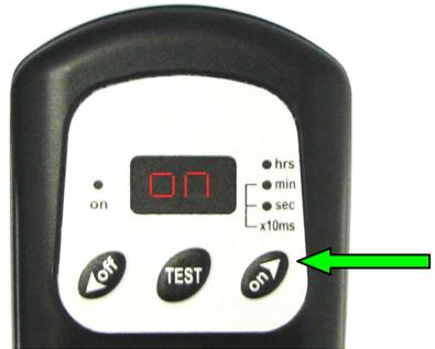
13. If the desired ON time is set, then simply don't press any buttons and after a few seconds the display will start flashing illustrating that the new time is being saved. Once the new time is saved, the unit will start operating with the new time setting.
